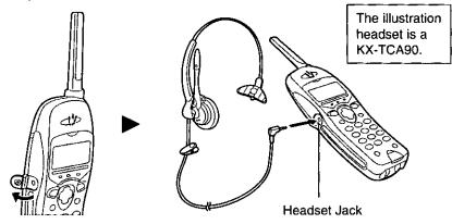
When an optional headset is connected to the handset, make sure to use the headset to talk with the caller. If you want to have a normal cordless phone conversation, disconnect the headset.
